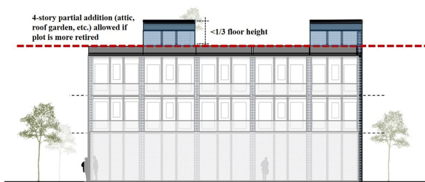
Fig. 6-7 Illustration of partial roof addition (Source: by the author)
