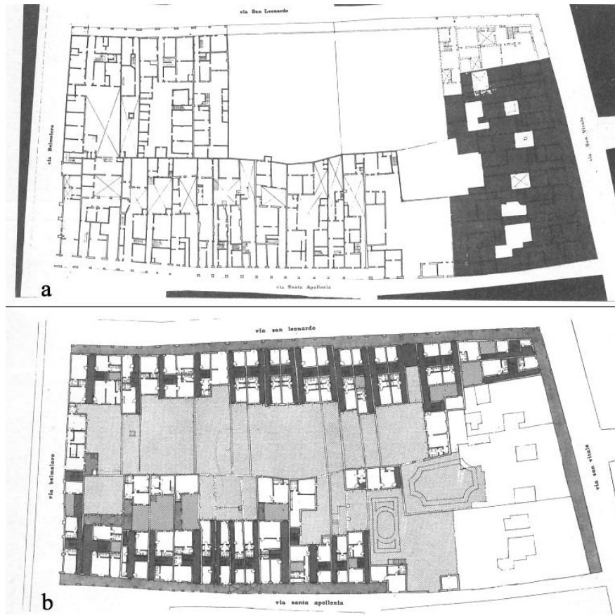
Fig. 2-18 Ground floor plan in S. Leonardo block C. a. Status plan; b. Design results
