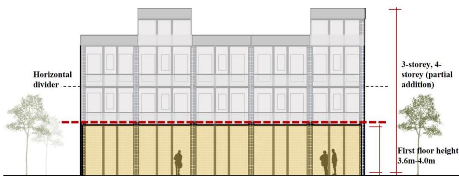
Fig. 6-8 Illustration of floor height and number of floors (Source: by the author)
