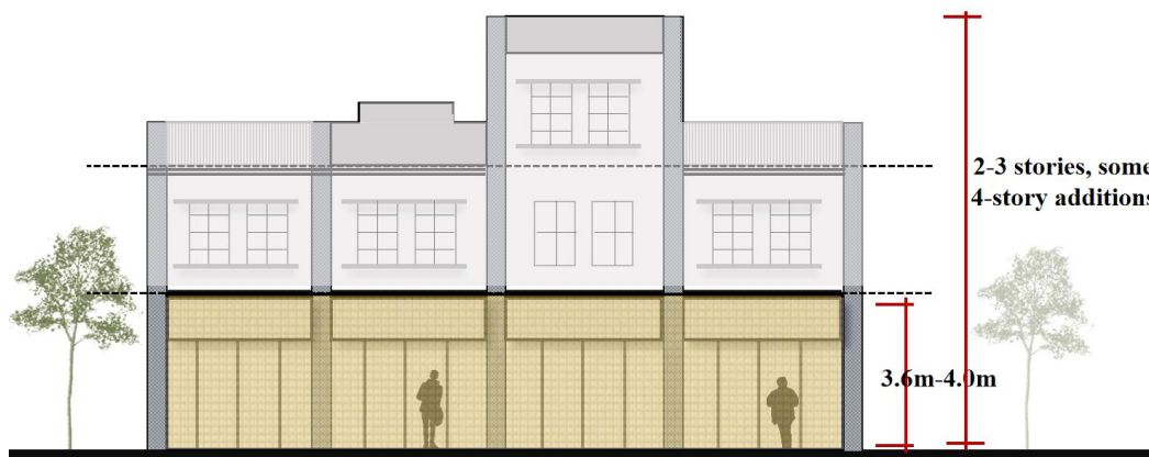
Fig. 6-19 Illustration of floor height and number of floors (Source: by the author)
