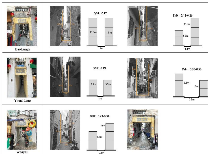
Fig. 4-11 Schematic results of D/H mapping of Class III streets and lanes (Source: by the author)
