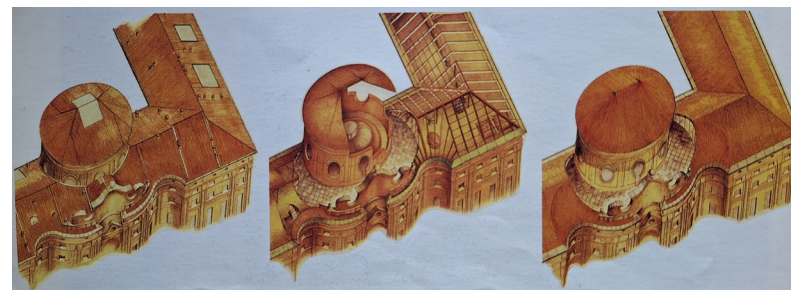
Fig. 3.12. Sketches illustrating the idea of freeing the roof of the XVIII c. wing by removing parts of it. Source: Mastropietro, Oltre il Restauro , 222.
