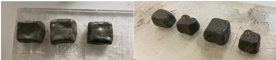
Image 23 Moldability test physical behavior results showing the evolution and variation of the mortars workability by creating different mis design formulations. Source: (Author)
