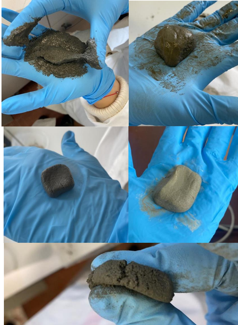
Image 21 Moldability and physical behavior test results of various mortar mix designs. Source: (Author)
