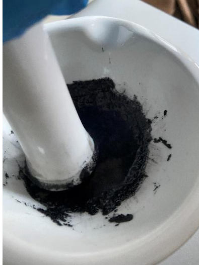
Image 11 Biochar hydrated pre grinding crushing process.
