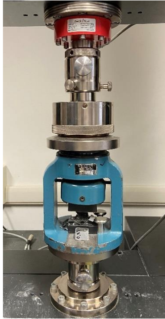
Image 47 Zwick Line-Z010 testing machine with the arrangement of compression fixtures. Source: (Author).
