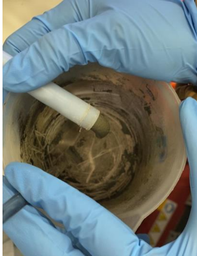
Image 30 Teflon tube mixture fluidity test. Source: (Author)
