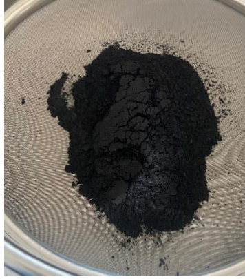
Image 13 Final biochar 250 \mu\text{m} particle size after sieving. Source: (Author)
