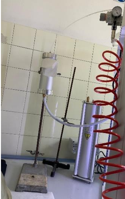
Image 28 tank placement setup and connection to the pressure compression and the Teflon tube Source: (Author).
