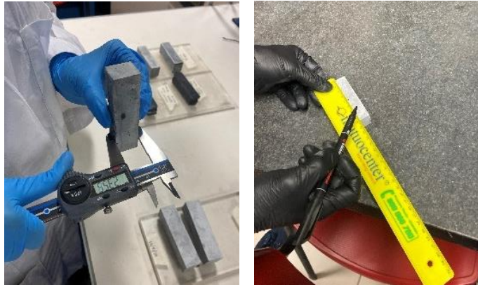
Image 44 Measurement of samples and marking referent points in preparation for the three-point bending test. Source: (Author).
