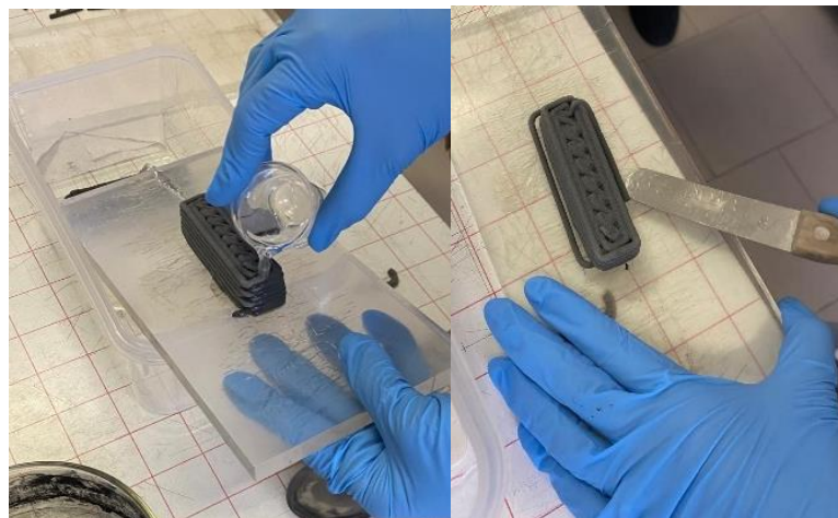
Image 38 Unmolding process of 3D printed samples. Source: (Author)
