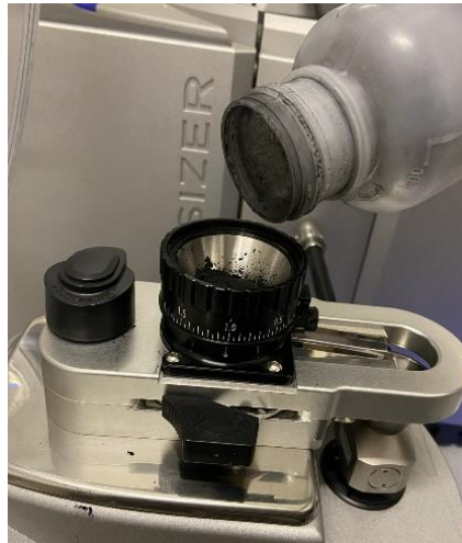
Image 124 Introducing biochar powder particles into the conical steel cell for granulometry analysis Source: (Author).
