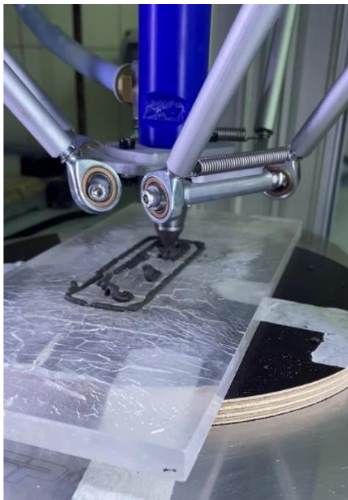
Image 32 3D printer, first printing layer problems due to nozzle blockage.
