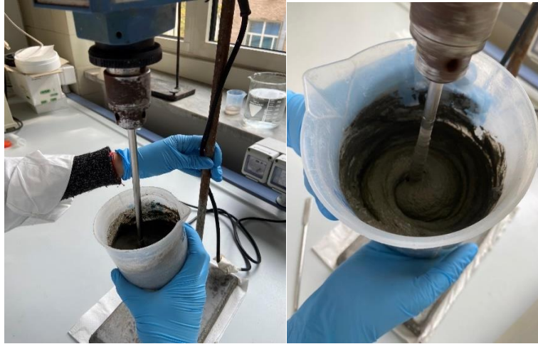
Image 17. mechanical mixture of all mortar mix design constituents. Source: (Author)
