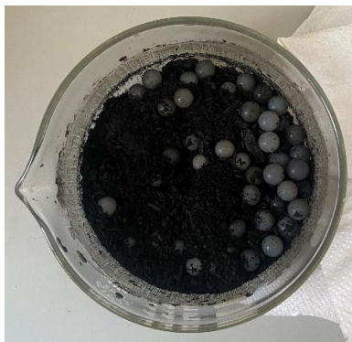
Image 12 Fully dried biochar after 48 hours.
