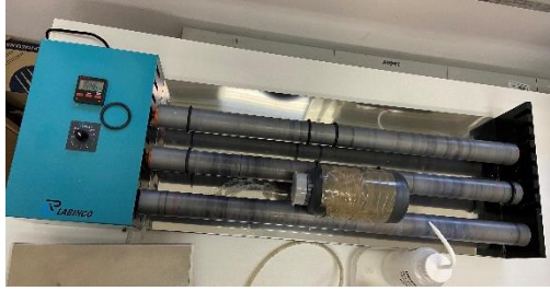
Image 9 Biochar grinding in the rolling bench. Source: (Author)
