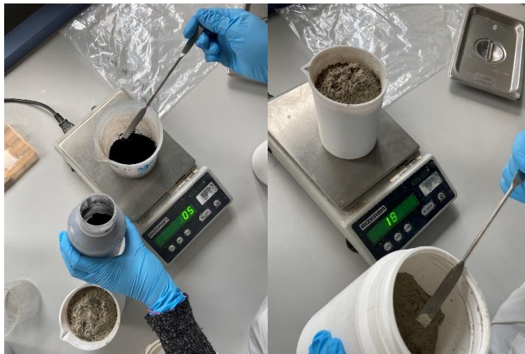
Image 16 Sand and mortar were already weighed, and biochar weighing is being carried out. Source: (Author)
