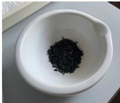
Image 10 Biochar after dry grinding, seamlessly change done to the particle size. Source: (Author)
