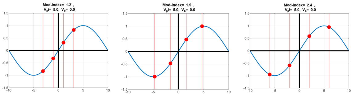
Figure 4.2: One quadrant of the 16QAM constellation displayed for different modulation indices.
