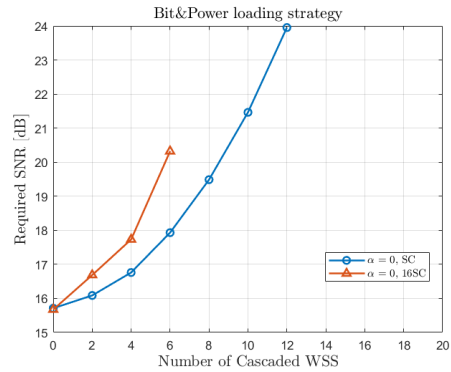
Figure 3.34: Required SNR [dB] vs. N_{WSS} with \alpha = 0 SC and \alpha = 0 16SCs for N_{WSS} \in \{0, \dots, 20\} , HD-FEC, Bit&Power Loading strategy
