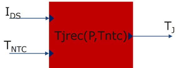
Figure 16 - 2 input, 1 output thermal model/function. (company slide 111)
