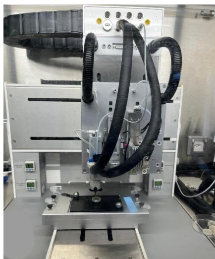
Figure 3.1 3D Discovery bioprinter during a sample printing.
