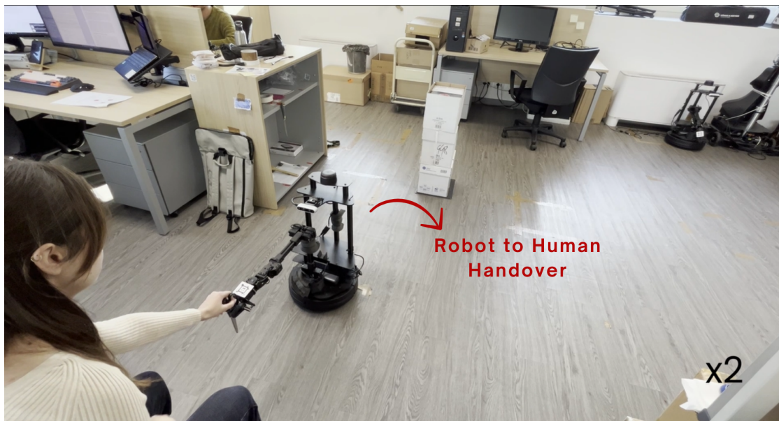
Figure 9.4: The Locobot comes back to the user and proceed with the handover maneuver
