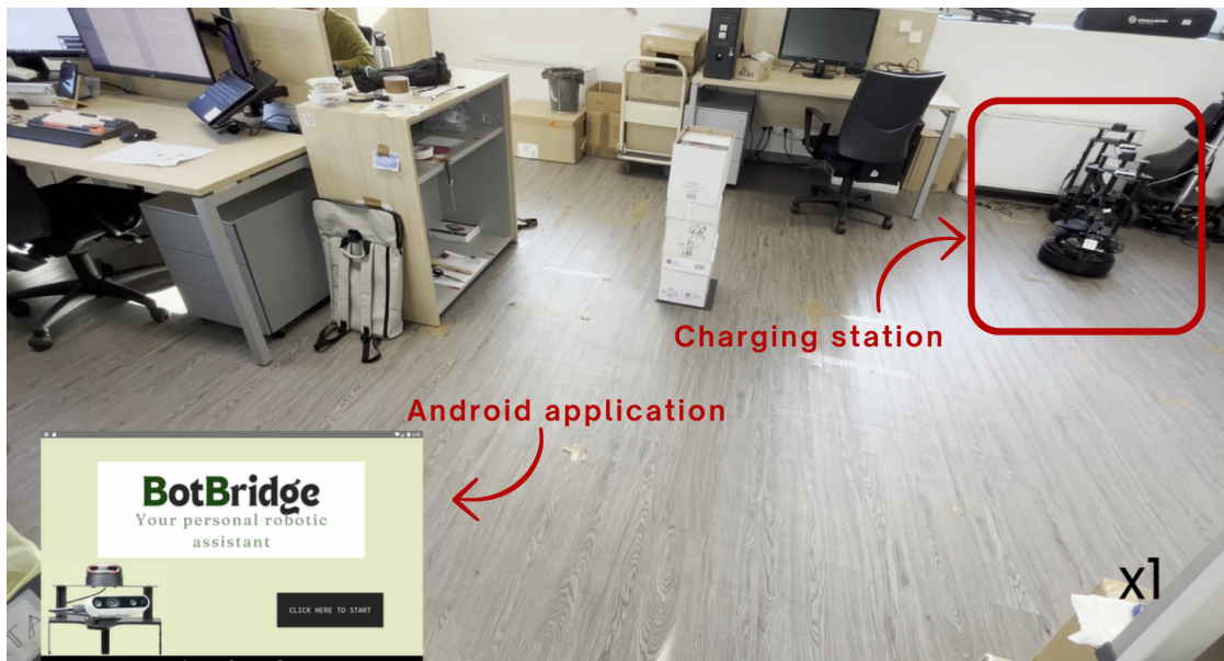
Figure 9.1: Starting situation with the robot at the charging station and the initial screen of the application in the bottom left
