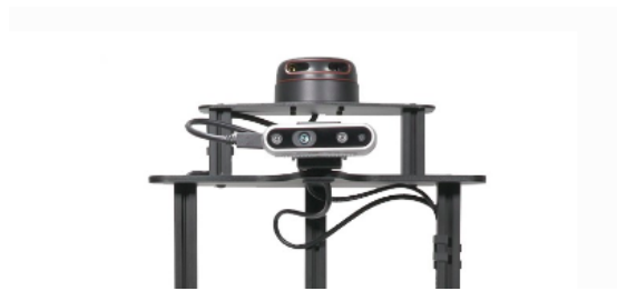
Figure 4.4: Locobot wx250 on board sensors [60]
