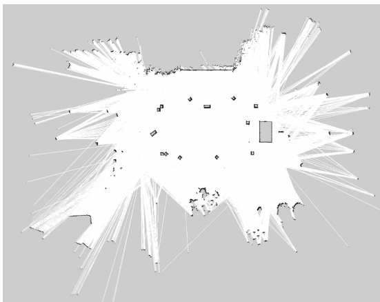
Figure 3.5: Mapping of the environment using gmapping package [52]
