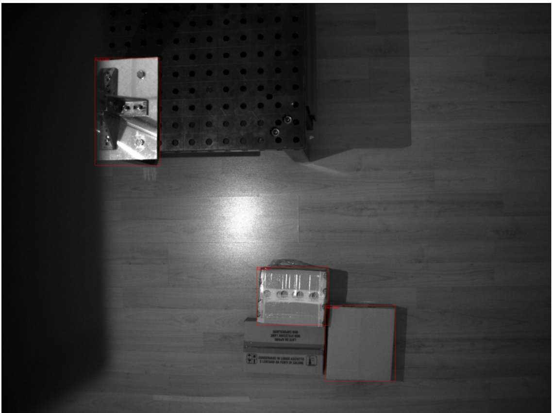
Figure 49 - Example 5 of object detection with a model trained with a mixed dataset. In top-left position the mount on the table is misclassified as a box
