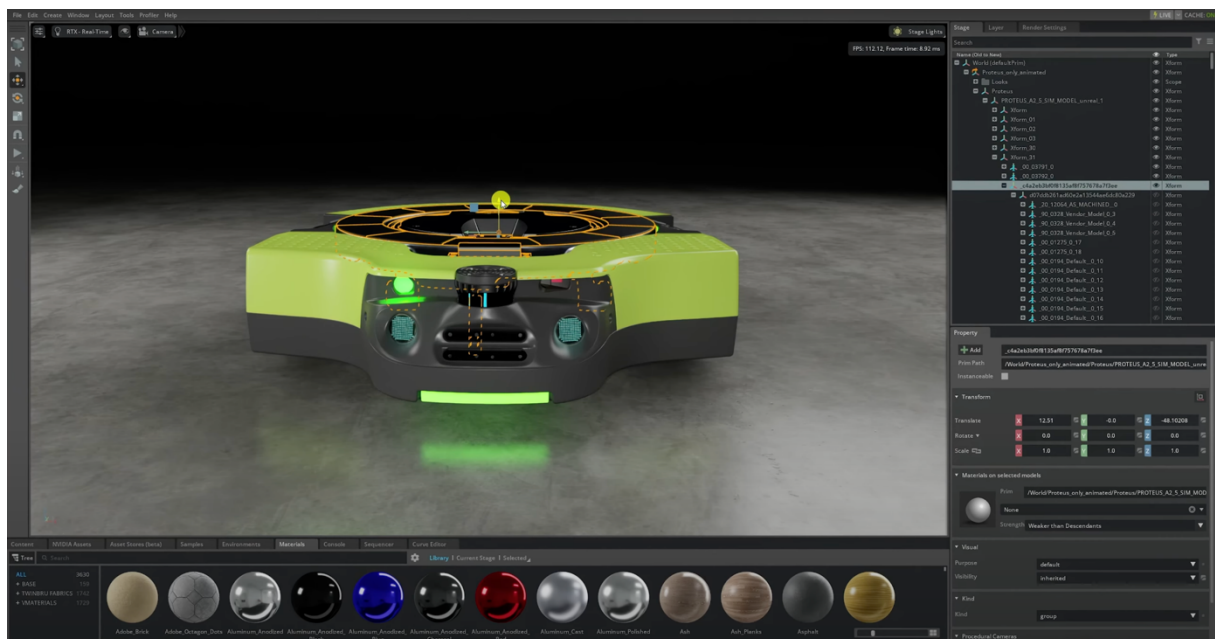
Figure 10 - Digital Twin of the Proteus Robot during a simulation in NVIDIA Isaac Sim 31
