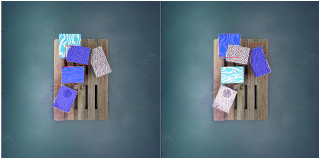
Figure 17 – Qualitatively example of object detection and instance segmentation with the model chosen. Blu areas are the segmentation masks, while red boxes are the bounding boxes.
