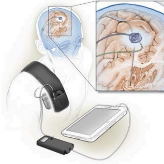
Figure 1.10: The figure shows a totally implanted bidirectional neural interface designed for chronic multisite recording in humans, as well as therapeutic neurostimulation [6].
