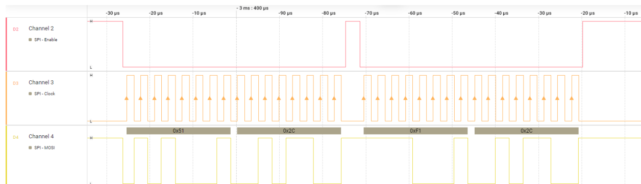
Figure 6-7 SPI communication signals captured from the real project and shows sending data to the MCP4922
