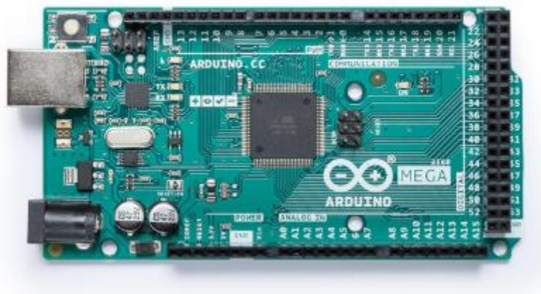
Figure 4: Arduino Mega2560 control board
