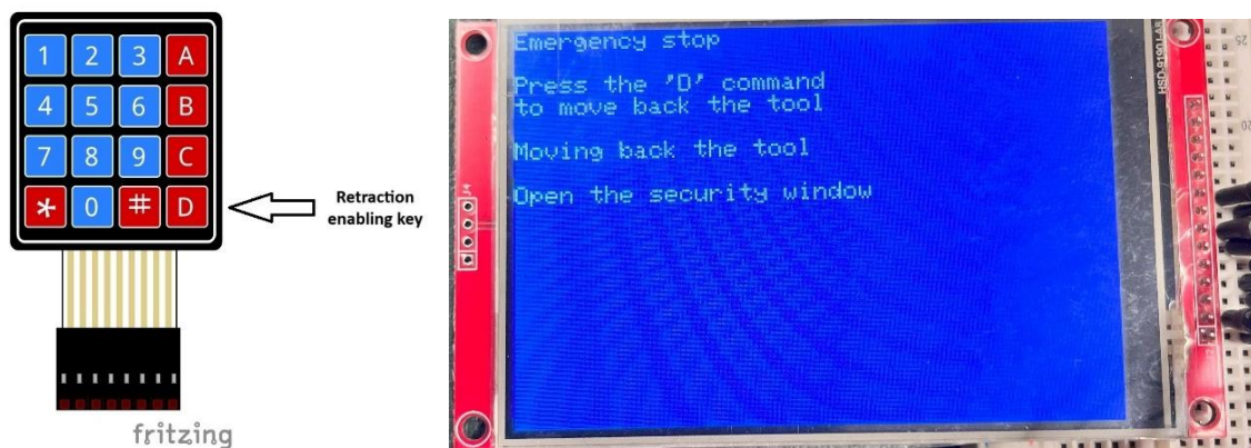
Figure 58: Key to enable the retraction of the tool and emergency stop operations
