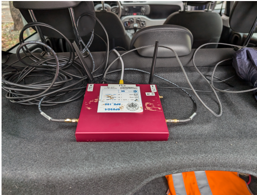
Figure 5.1: OBU installed in vehicle
