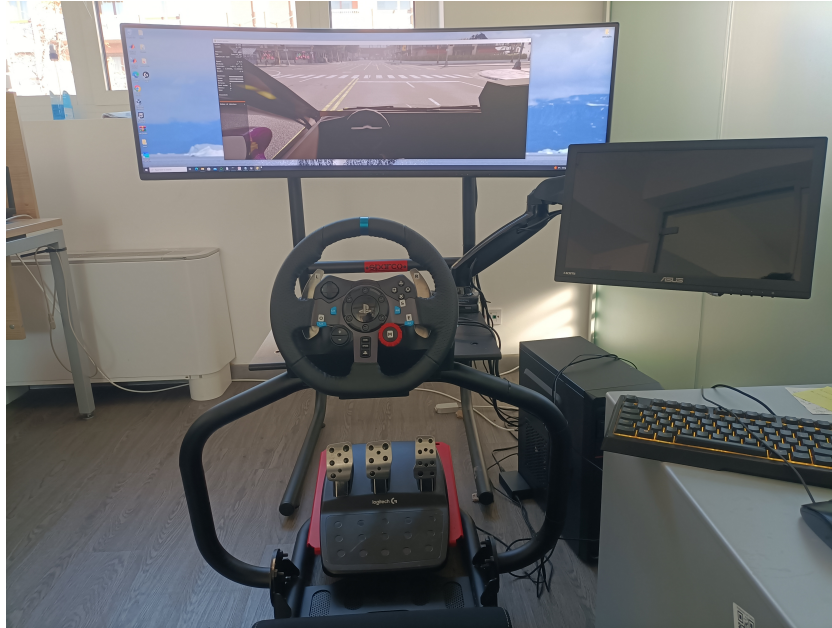
Figure 3.5: Steering wheel and pedals setup for manual driving
