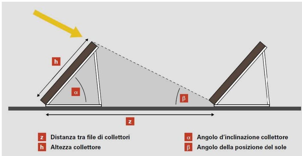
Figure 3-3 Flat roof installation (Source: Viessmann manuale solare completo)
