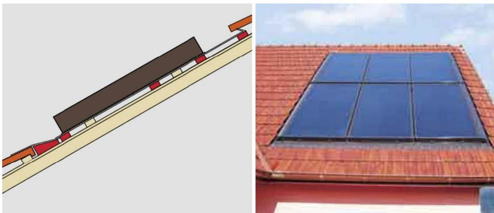
Figure 3-4 Installation method of photovoltaic panels on slope roof (Source: Viessmann manuale solare completo)
