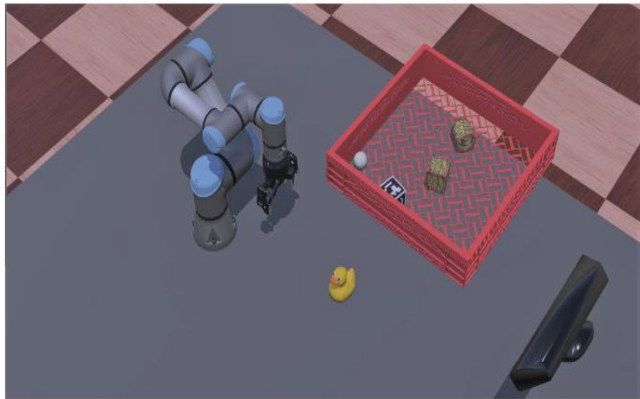
Figure 12 The virtual environment built on Webots: it consists of a table, a UR3e cobot (left) with a two-finger gripper, an RGBD camera (right) and the objects to be manipulated by the robot [11].
