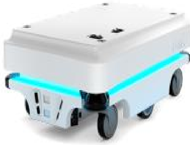
Figure 14 MiR100 Mobile Robot [21]
