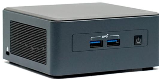
NUC (abbreviation for Next Unit of Computing) is a family of compact computers developed by Intel and then by ASUS. They are characterized by their light weight and smaller physical size with respect to other kinds of computers with similar features and are thus feasible for usage on medium-sized mobile robots requiring computational power comparable to laptops. The model on which development
