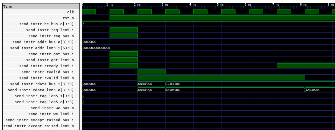
Figure 4.2: Execution of an Instruction Request and Response with Ready Signal Deassertion
