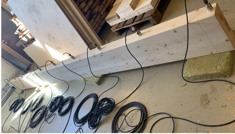
Figure 8.2: Photo of the experimental setup conducted on the timber beam dynamic identification application.
