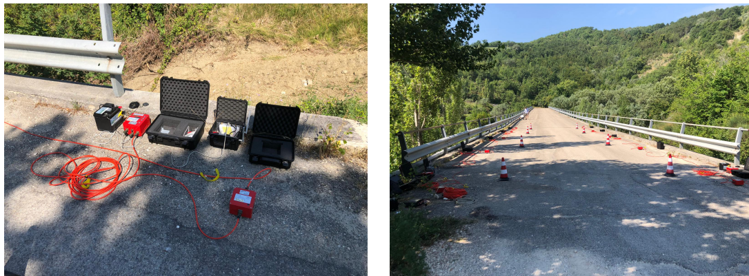
Figure 8.12: Corvara bridge case study: wired data acquisition setup.
