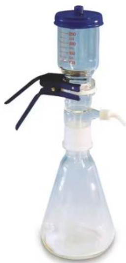
Figure 2.5 Filtration glass vacuum device. The white tube on the right allows connection to the pump to create vacuum.
