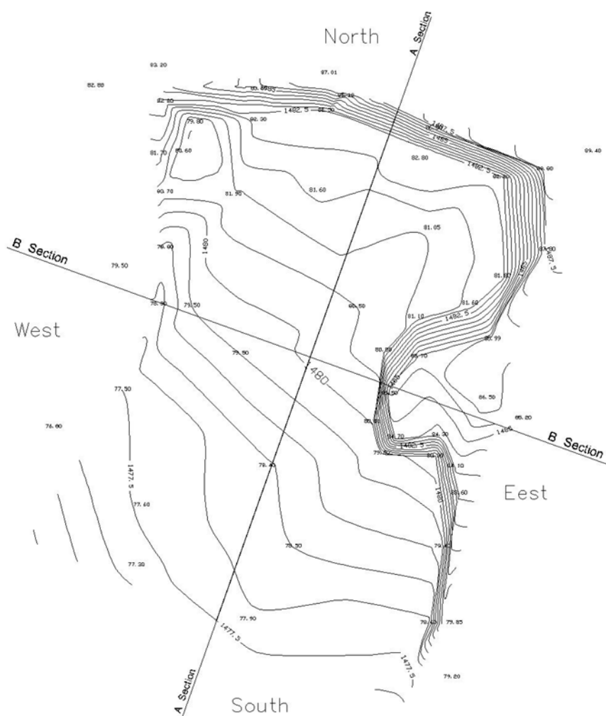
Figure 61: Displays the topography, slope direction, and elevation differences, offering a detailed view of the natural layout of the site (Novin Shahrzaz, 2020).
