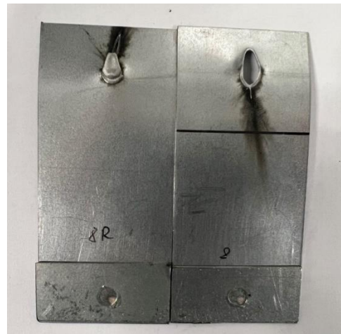
Figure 22- Specimen affected by expulsion.
