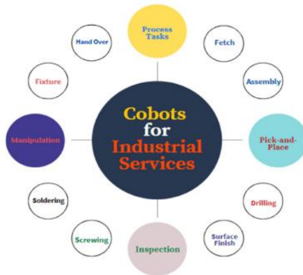
Figure 17 - Possible Collaborative Robots applications in Manufacturing. [61]
