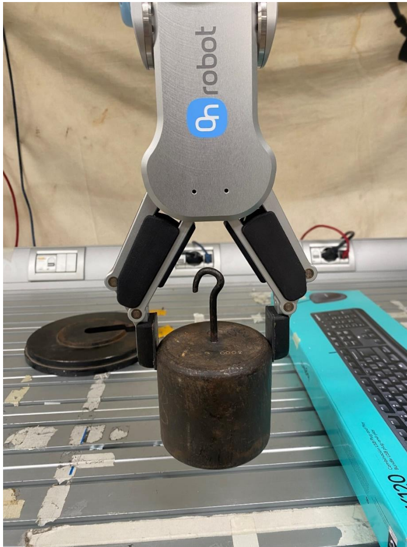
Figure 23 - 3kg payload transported by the UR3e collaborative robots.
