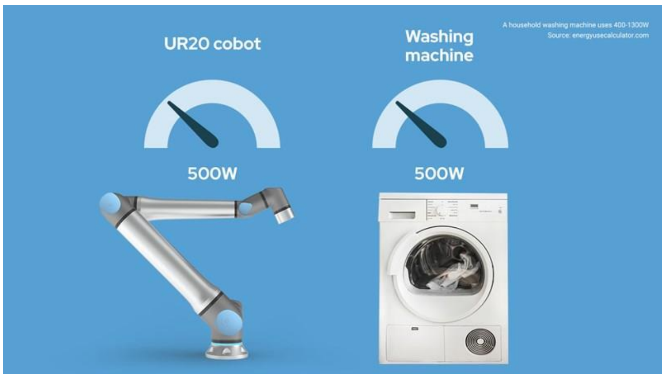
Figure 22 - Comparison among the energy consumed by the UR20e cobots and a washing machine [83]
