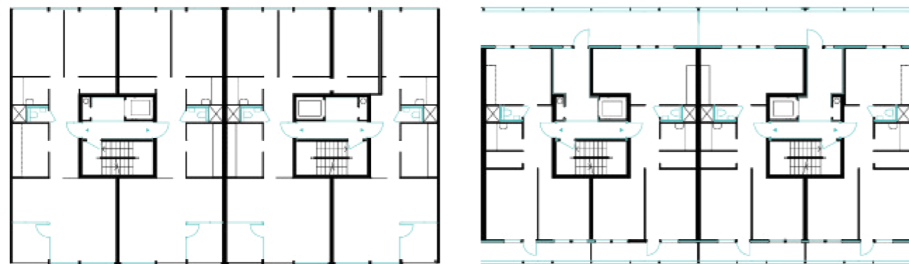
Figure 2.13: Change in floor plans highlighted in blue in regular floor plan and communal corridor floor plan (6)
