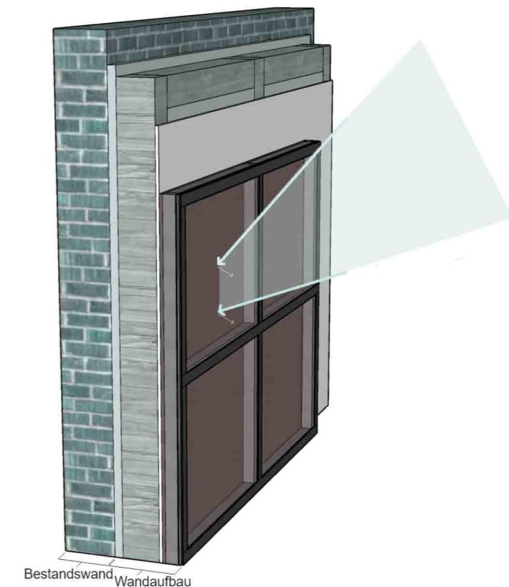
Figure 2.32: Trombe wall façade with honeycomb cardboard filling (18)
