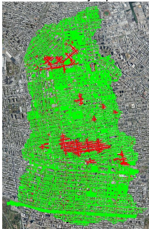
Figure 68: Map of instability BIRR case for vehicles. Red areas are zones of instability that induce the movement of the cars. Green areas are zones of stability
