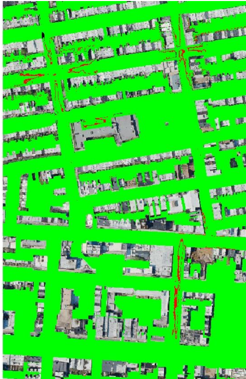
Figure 79: Focus map of instability variations for people, (BIRR+RC)-Baseline. In this case respect to the BIRR-Baseline case for people with coupling with the RC methods there is a reduction of the vulnerability respect to the baseline as visible from the red areas.
