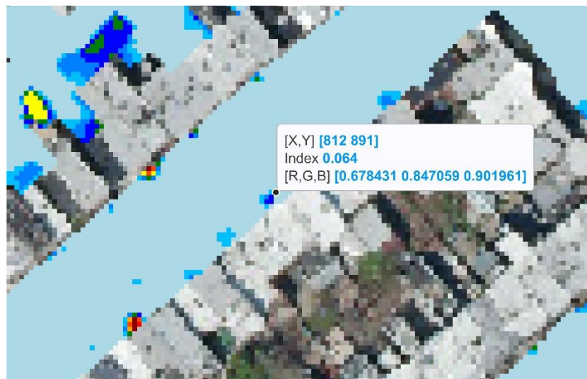
Figure 64: Focus cell value around the downspout. The downspout presence is characterized by a circular area adjacent to the edge of the area of the building.
