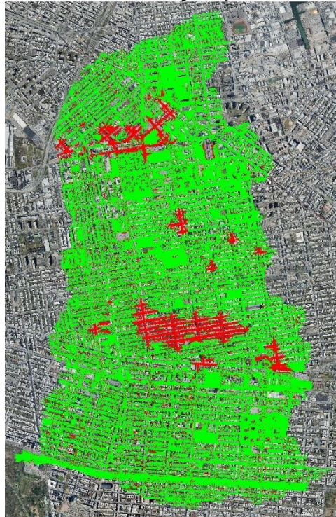
Figure 67: Map of instability Baseline case for vehicles. Red areas are zones of instability that induce the movement of the cars. Green areas are zones of stability
