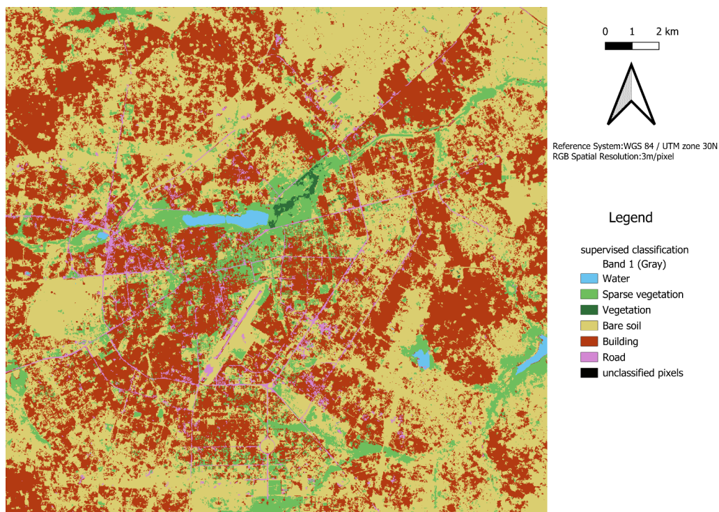
Figure 35. The Classification of Test 7( This map displays the results of the supervised classification using manually selected training samples. The classification differentiates between water, bare soil, buildings, roads, sparse vegetation, and dense vegetation, reflecting the land cover distribution in Ouagadougou.)
