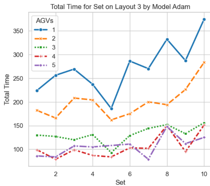
Description: This graph shows the evolution of total time for each set based on the amount of AGVs on layout 3.
