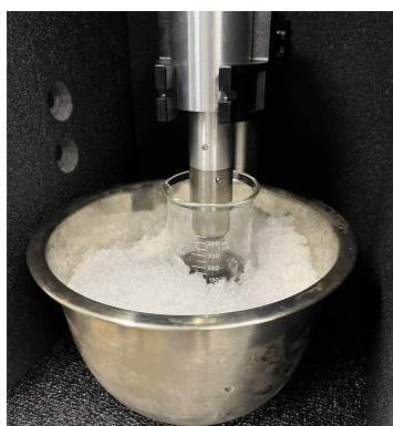
Figure 3.5: Sonicator working at a frequency between 20 and 40 kHz.
