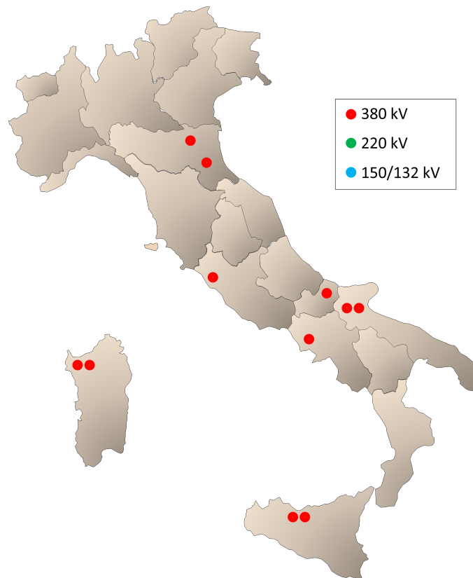
Figure 2.5: Synchronous condensers that are planned to be installed in the coming years. [Source: Terna]
