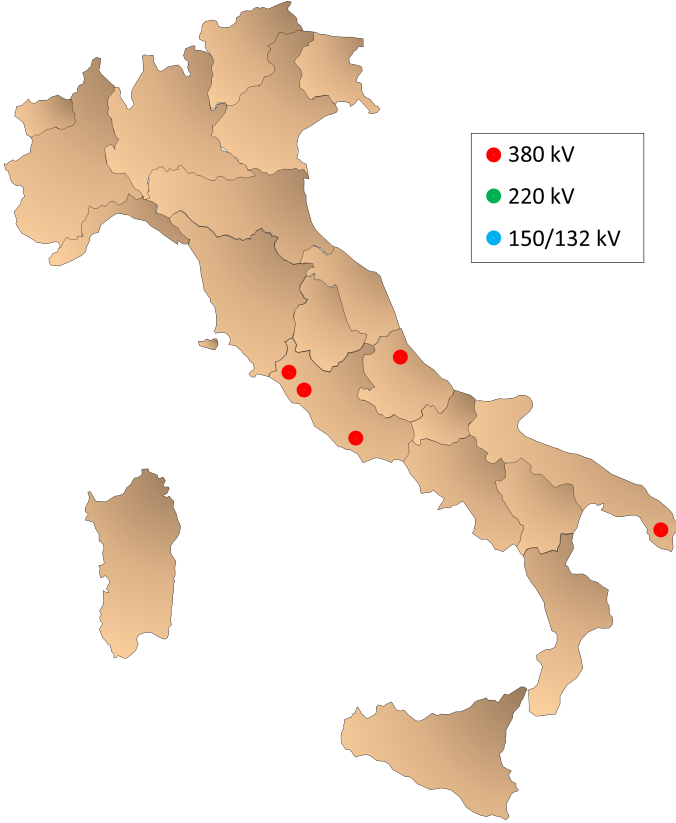
Figure 2.10: Geographical distribution of the installed STATCOMs. [Source: Terna]
