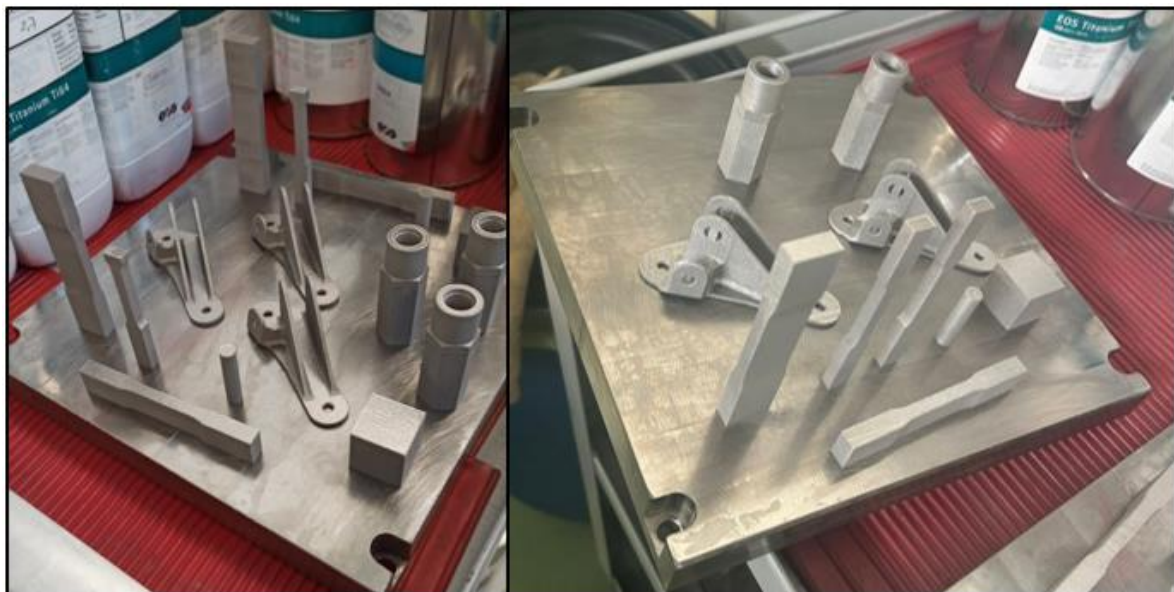
Figure 2.12 – Ti6Al4V job 1 built with steel recoater (left) & job 2 built with carbon fibers recoater (right).
