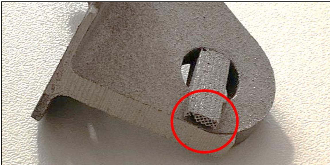
Figure 2.9 – Lattice support on C-27J Bracket.
