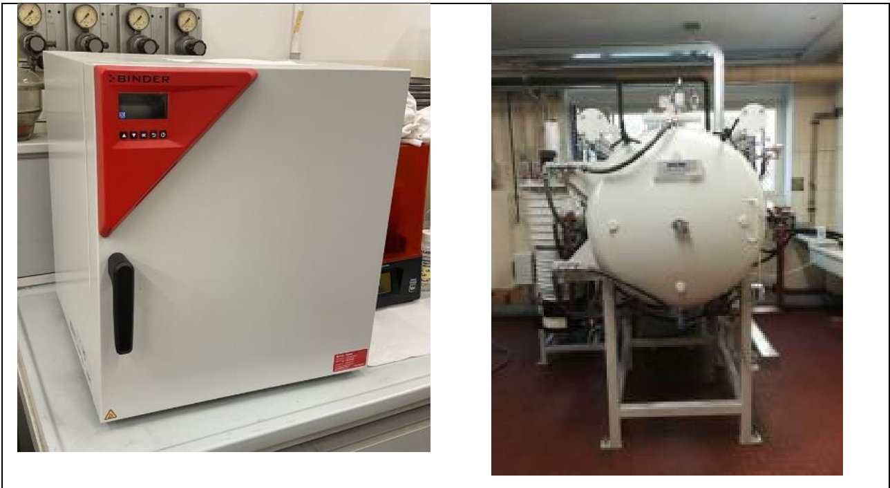
Figure 2.13 – Heating chamber (left) & Pro.ba furnace used for vacuum heat treatment (right).
