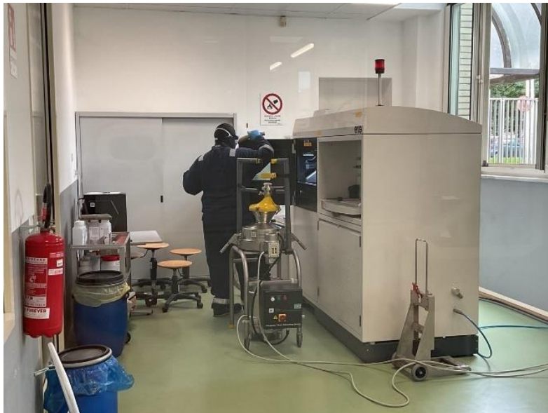
Figure 1.13 – Process of loading the LPBF machine.
