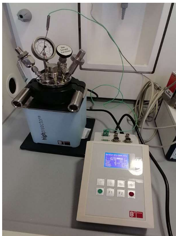
Figure 20: Transfer of the mixture into the autoclave chamber, consisting of three components: the hydrothermal bath, the heater, and the thermocouple.
