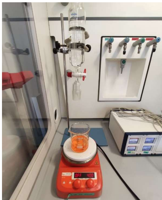
Figure 17: Dropwise addition of Solution B into Solution A using a dropping funnel, while constant stirring is maintained with a magnet at 400 rpm.
