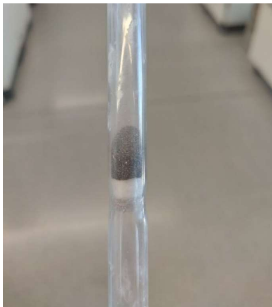
Figure 25: Quartz reactor showing a fixed bed composed of foam support, a quartz wool layer, and a silicon carbide catalytic bed with a nickel monometallic catalyst.
