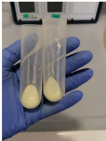
Figure 19: \text{CeO}_2 nanoparticles settle at the bottom of centrifuge tubes after centrifugation and liquid separation.
