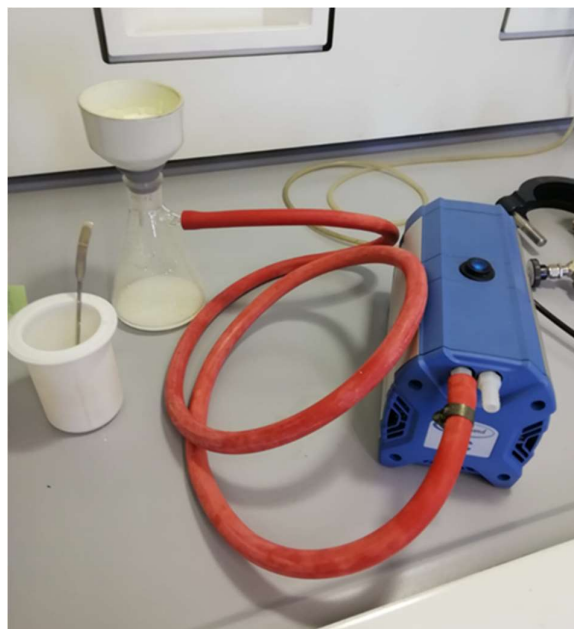
Figure 21: Filtration process using a ceramic filter connected to a pump and a Kitasato flask, with filter paper inserted, to separate the solvent from the synthesized material.
