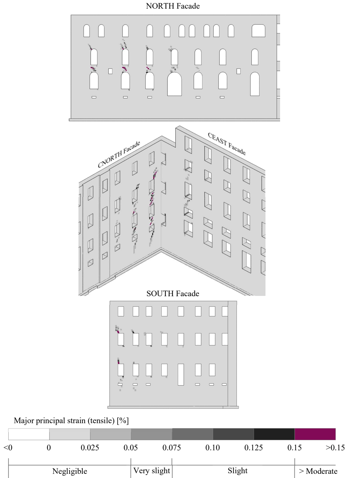
Figure 6.102. Interaction model: Major principal strains of the individual facades for the INT_VLMIN condition with CDP MAX masonry constitutive behavior
