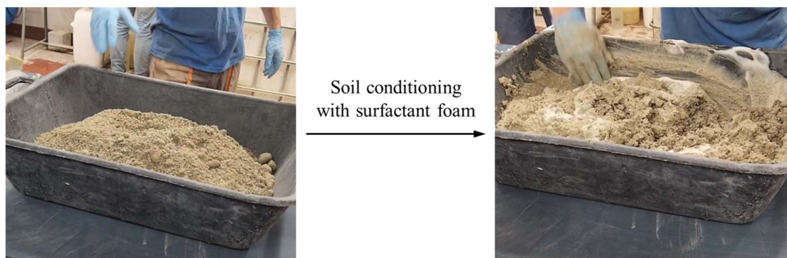
Figure 2.4. Emulation of the soil conditioning of an EPB-TBM
