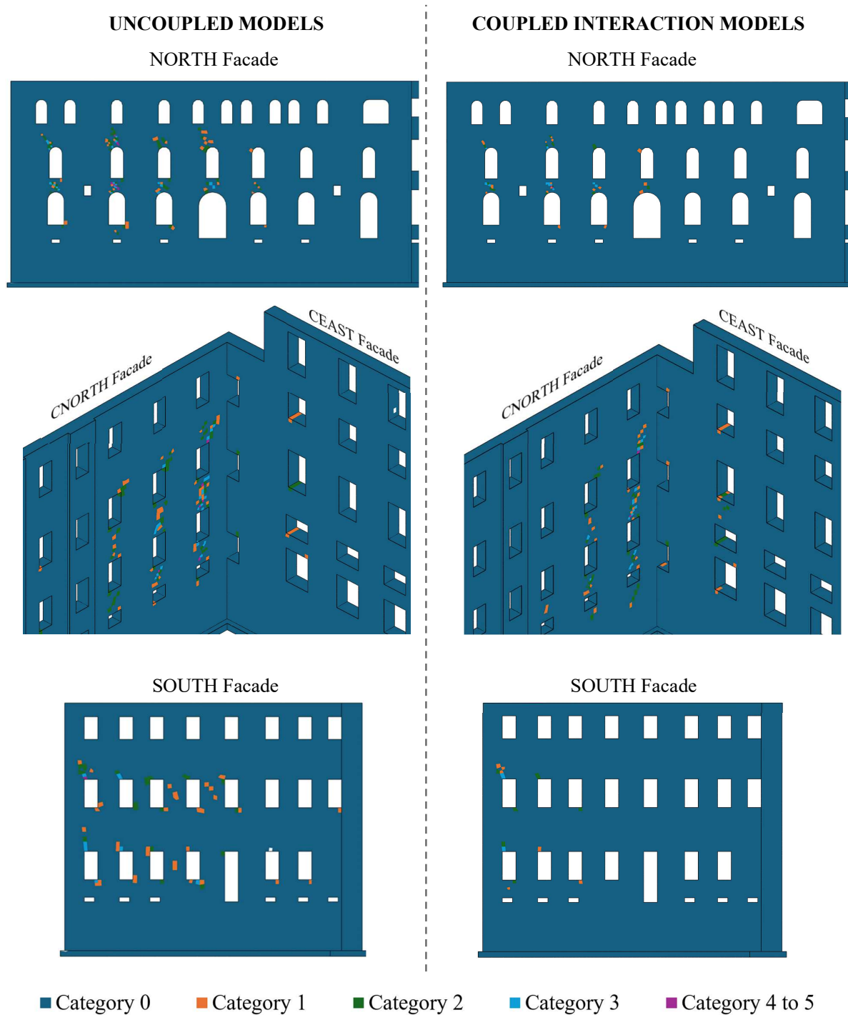
Figure 6.105. Comparison of damage category maps between individual facades of the uncoupled and coupled interaction models, for the VLMIN condition with CDP MAX masonry constitutive behavior
