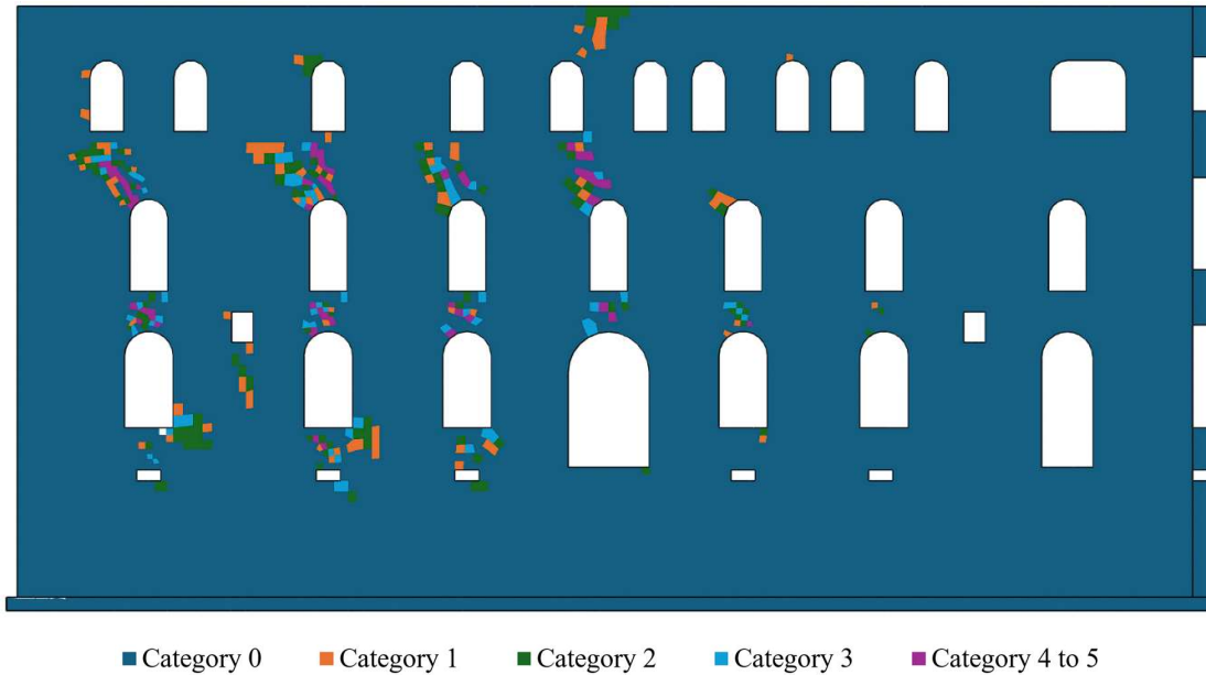
Figure 6.50. Uncoupled model: Damage category map of the NORTH facade for the VLMAX models with the CDP MAX masonry constitutive behavior
