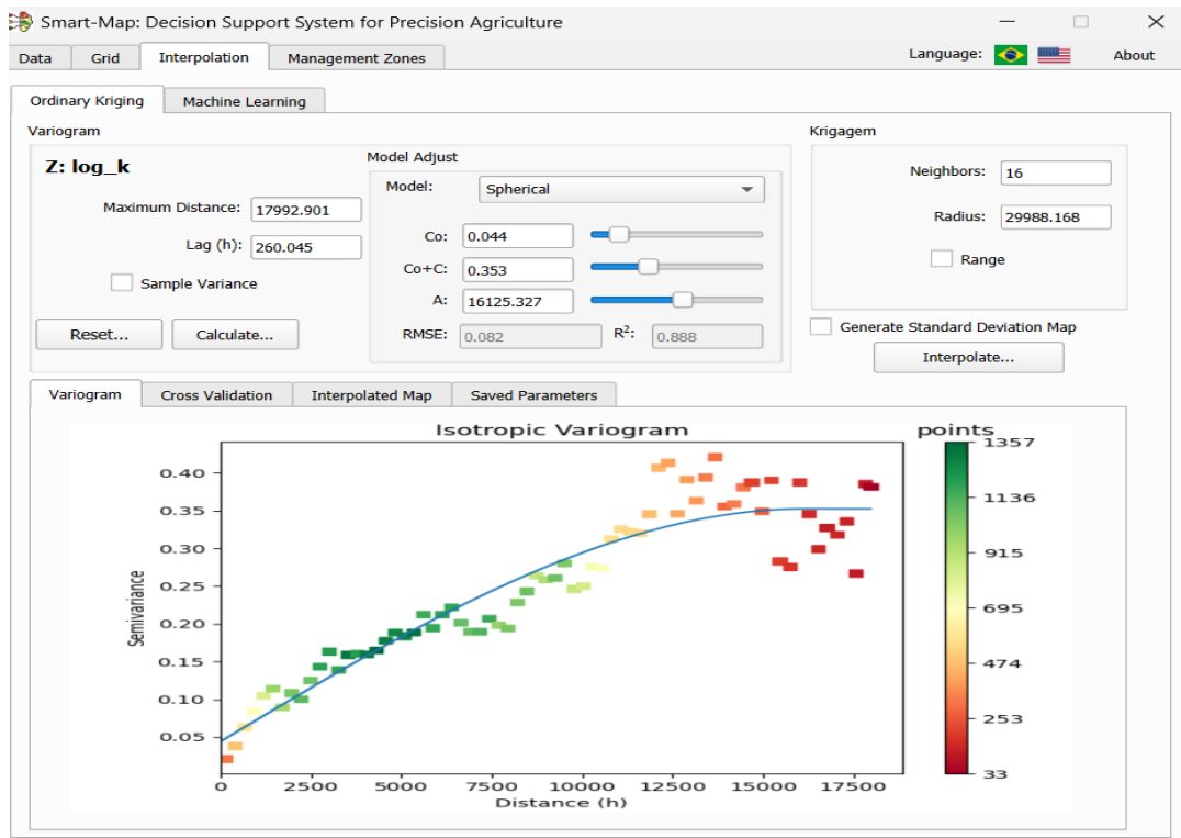
Fig. 9. Best fit for hydraulic conductivity: Spherical model
