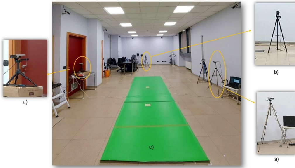
Figure 3.1.1: The experimental setup in the laboratory of the Polytechnic of Turin with a) Azure Kinect sensors, b) Vicon VUE camera, and c) green carpet.
