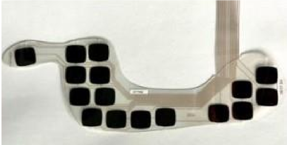
Figure 2.2.2.2.2: Illustration of a pressure insole with 16 sensing elements [20].
