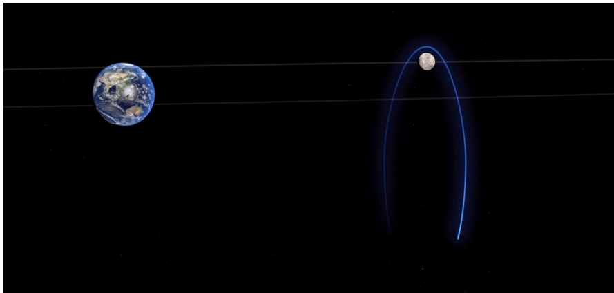
Figure 2.11: Gateway's near-rectilinear halo orbit, or NRHO, around the Moon, (Image credit: NASA)
