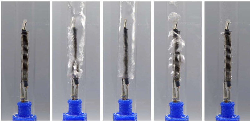
Figure 8: Heating of the coil under water demonstrating subcooling and pool boiling. [19]
