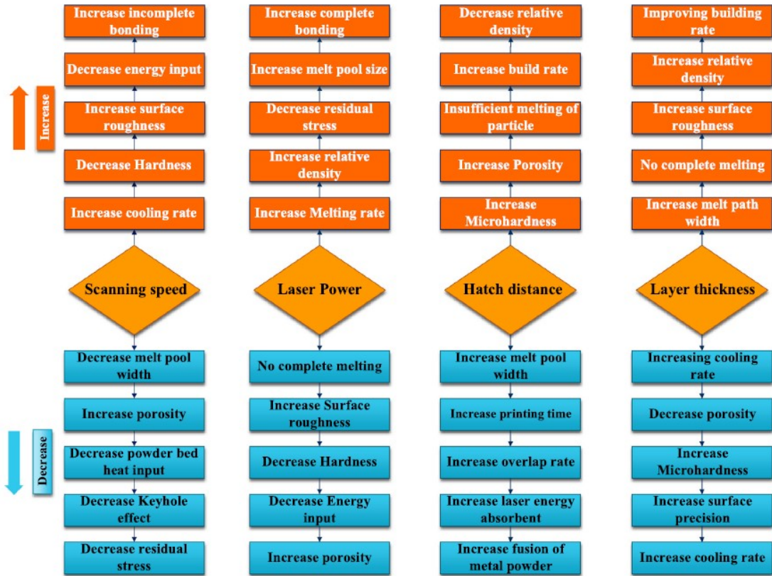
Figure 3.5: Effect of SLM process parameters [46]
