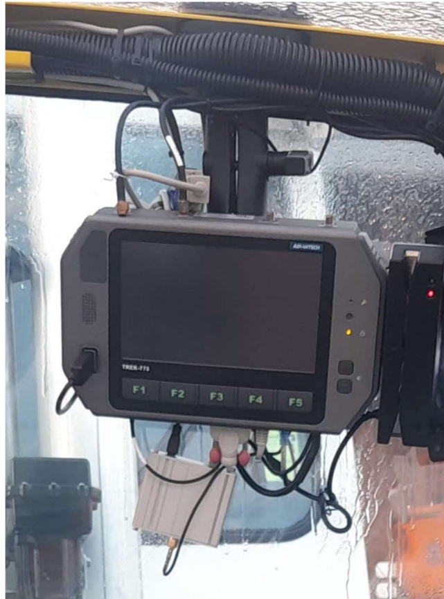
Fig. 5.2: Tablet through which informations are communicated to the de-icing operator.
