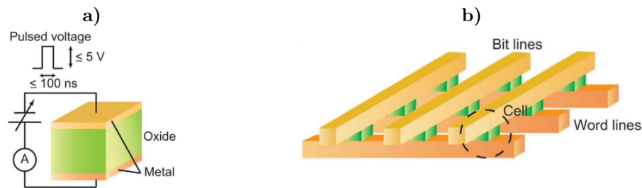
Figure 14: a) Schematic of a single ReRAM cell with applied voltage. b) Organization of ReRAM cells into a crosspoint memory array ensuring high-density and low-power storage. Word lines and bit lines are utilized for selecting a memory cell as well as for writing and reading data. Adapted from [31]
