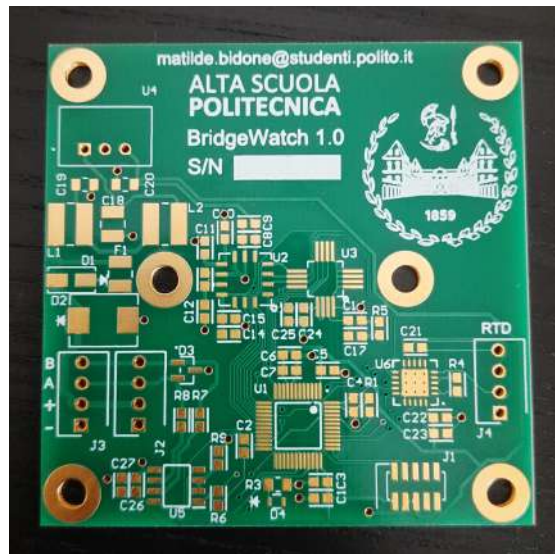
Figure 6.9: BridgeWatch board without components
