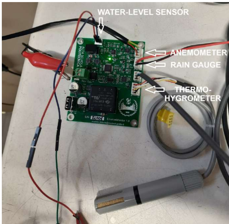
Figure 10.38: All sensors connected to EnvironMonitor board
