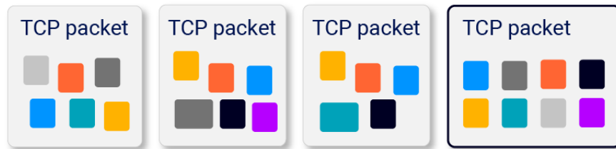
Figure 3.5: A closer look to the SPA: the last TCP packet contains the last bytes of every previous request. [29]
