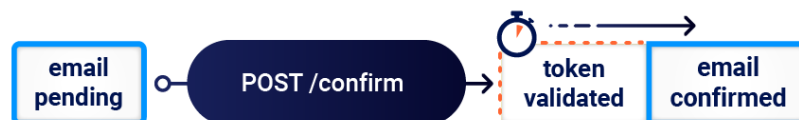
Figure 3.6: A scheme to visualize how GitLab verifies an email address through the use of a token. [29]
