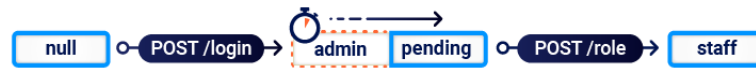
Figure 3.3: A multi-step sequence: the user is an admin for a few seconds, giving the possibility for unauthorized admin access. [29]
