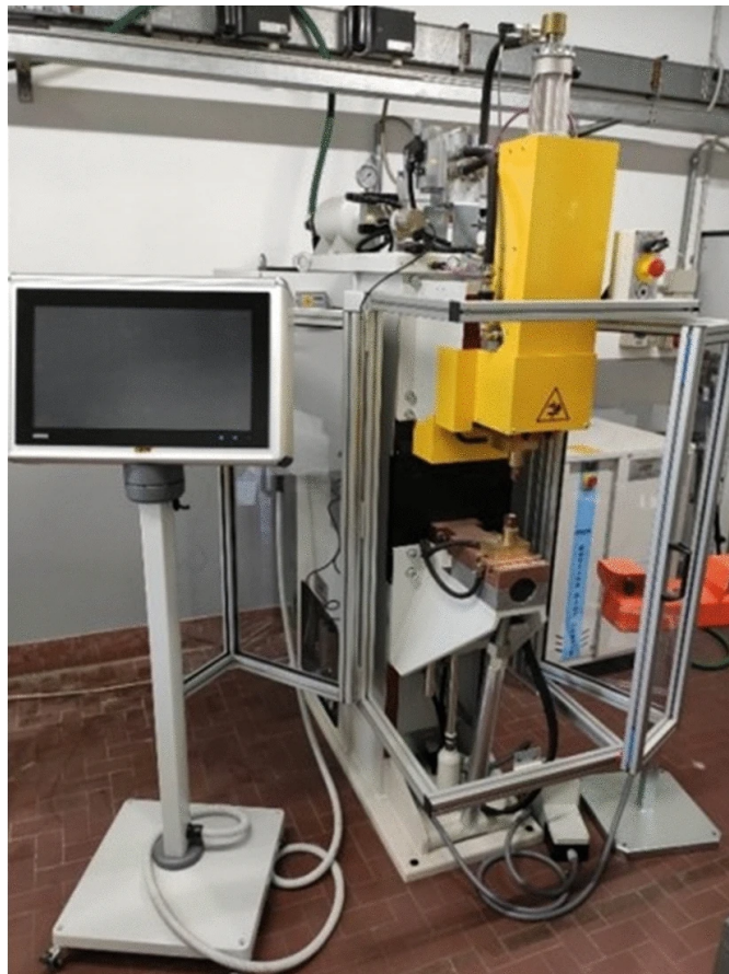
Figure 3.1: The Resistance Spot Welding Machine used for the experimental campaign[35]
