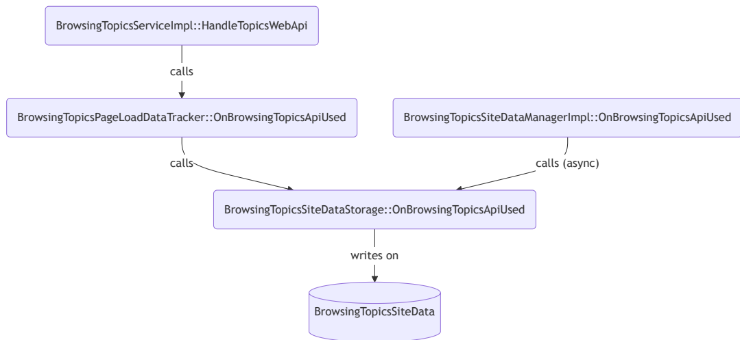
Figure 4.3: Dependency graph of functions that call OnBrowsingTopicsApiUsed and were modified for the purpose of this analysis.
