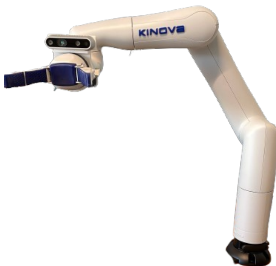
Figure 4.3: Setup of Kinova Gen. 3 Lite Manipulator with Intel RealSense D435i
