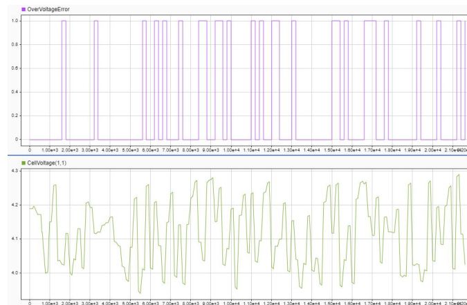
Figure 4.12. Overvoltage logic signal and cell voltage curve
