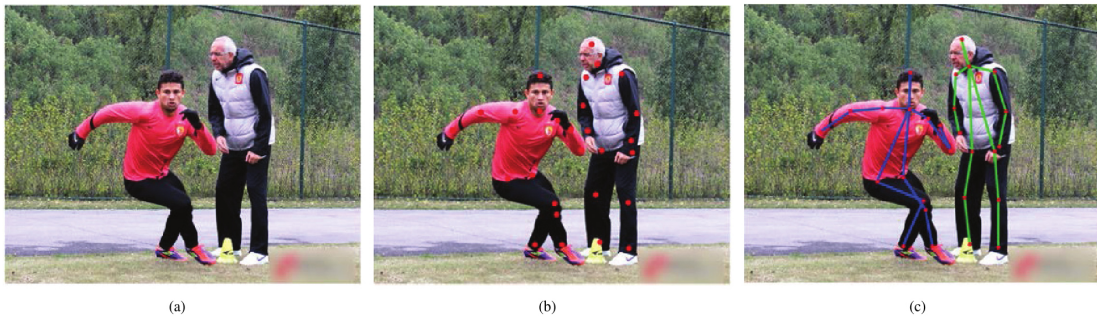
Figure 1.3: An illustration of bottom-up pipeline. (a) Input image, (b) keypoints of all the person, and (c) all detected keypoints are connected to form human instance [25].
