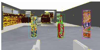
Figure 5.10: Object Recognition using the type-based policy.
