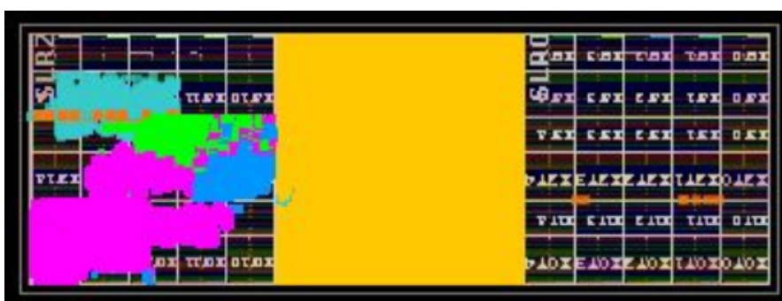
Figure 4.6: Area breakdown showing the contributions of Ariane processor and ITA accelerator in FPGA deployment.
