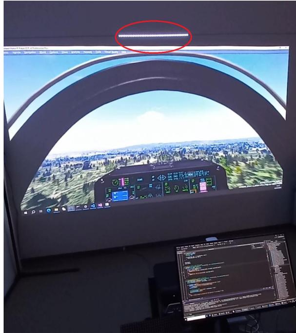
Figure 5.2: LED strip in no roll situation.
