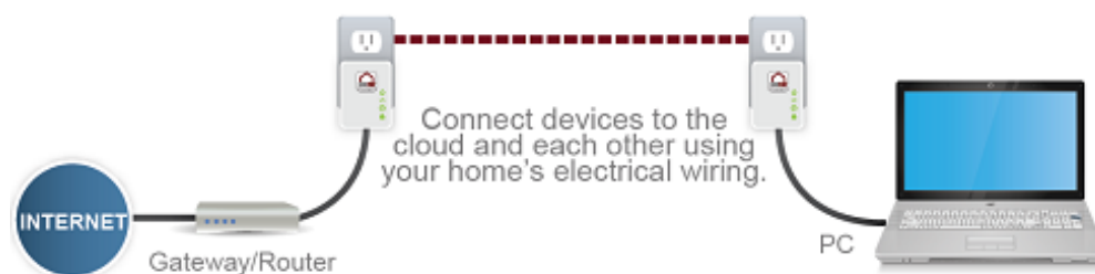
Figure 2.1: Network connection through a PLC (taken from [6])
